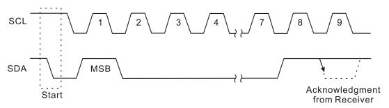
The audio processor that has been addressed has to generate an Acknowledge after receiving each byte; otherwise, the SDA Line will remain at the High Level during the ninth (9th) Clock Pulse. In this case, the master transmitter can generate the STOP Information in order to abort the transfer.
