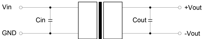
Figure 1. Typical external circuit
